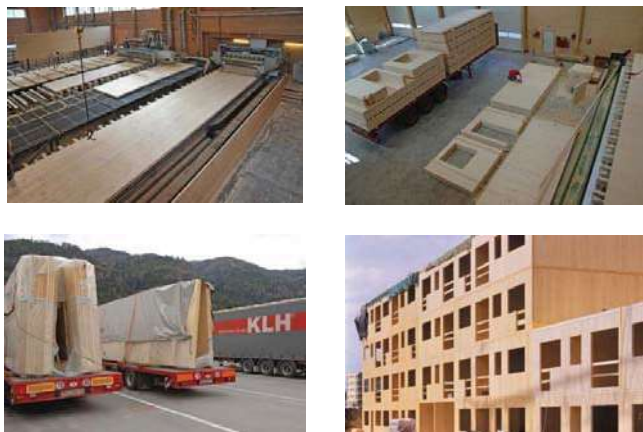
Figure 2. Manufacture, transportation and erection of CLT panels [Images: KLH].
