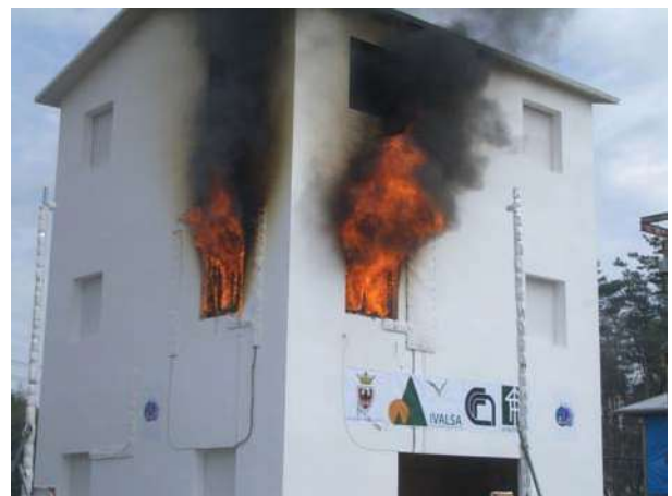
Figure 10. Fire test on 3-storey CLT building [24]
