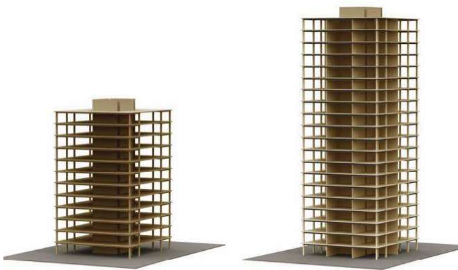
Figure 19. FFTT building frames: Options 1(12-storey) & 2 (20-storey) [30].
