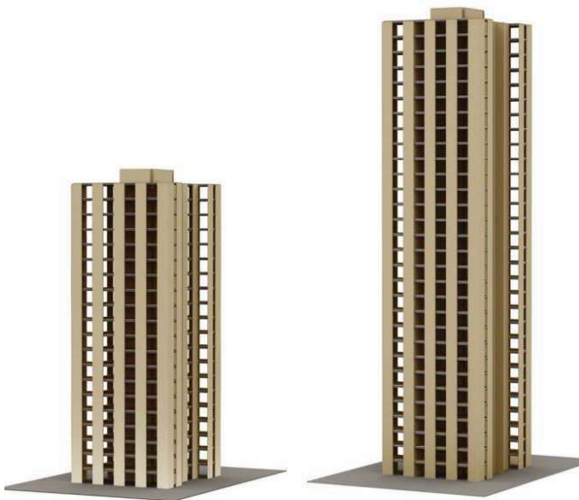
Figure 20. FFTT building frames: Options 3 (20-storey) & 4 (30-storey) [30].
