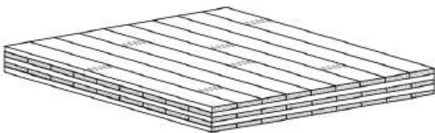
Figure 1. Five layer CLT panel [2].
