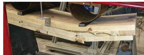
Figure 26. Rolling shear failure of Irish CLT panel
