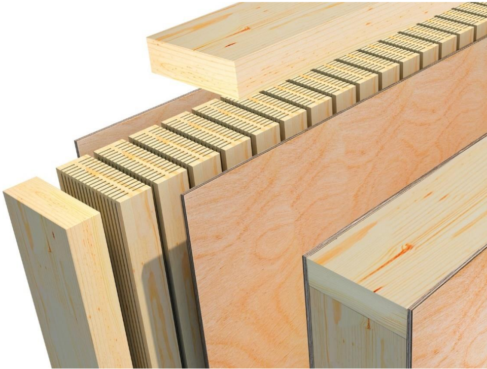
Figure 3.9 IsoTimber block composition: studs with air ducts placed next to each other, vertical plywood boards glued on each of the large sides (IsoTimber 2018)
