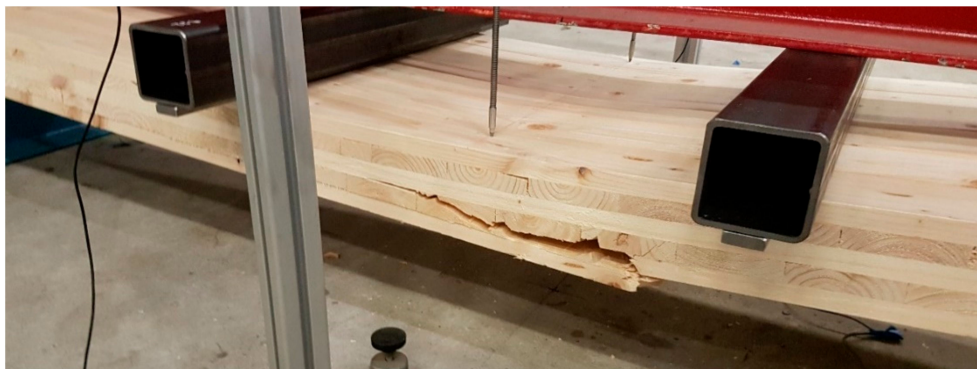
Figure 3. Bending failure on the bottom tensile face of the panel (B-5-20-7).
