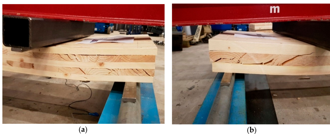
Figure 8. Rolling shear failure: (a) five-layer panel (S-5-20-5) and (b) three-layer panel (S-3-40-7).
