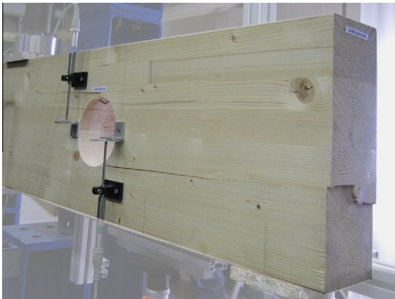
Fig. 14. Shear failure at holes.
